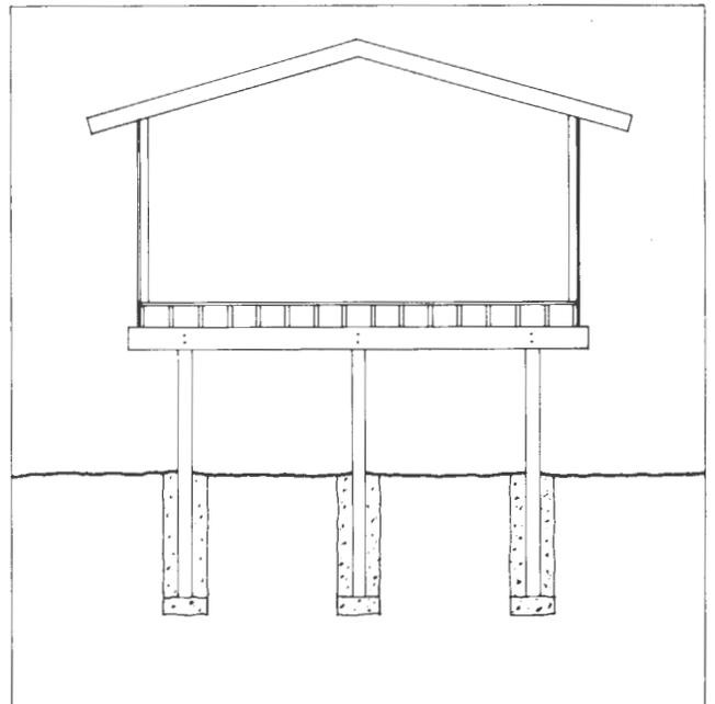
Figure 4.28. Platform Construction
