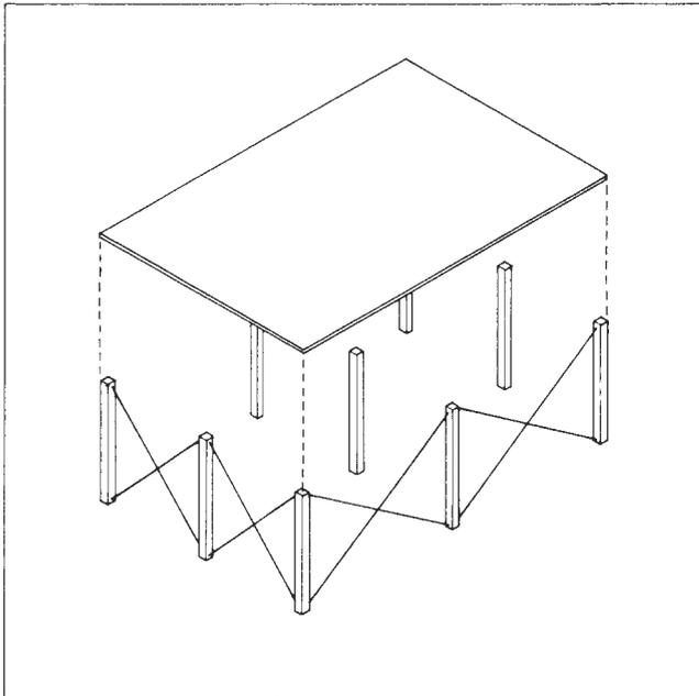
Figure 4.22. Diagonal Bracing
