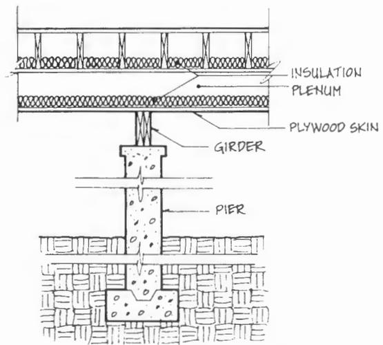
Figure 4.53. Double-Insulated Floor Plenum, Pier Foundation
