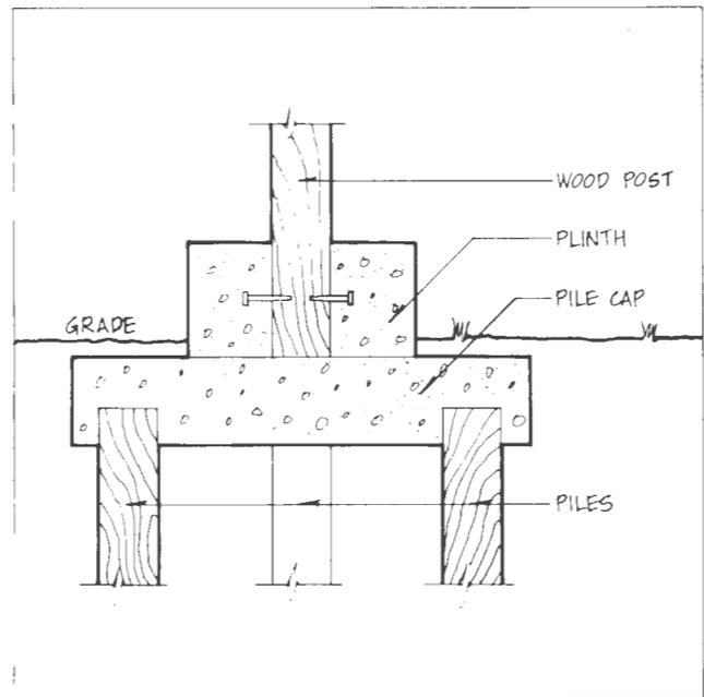
Figure 4.8. Post/Pile Foundation
