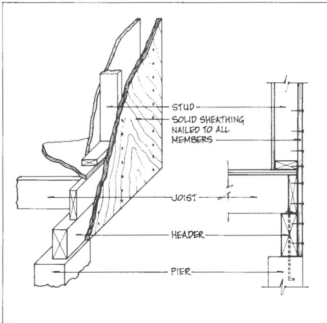
Figure 4.45. Plywood Anchorage
