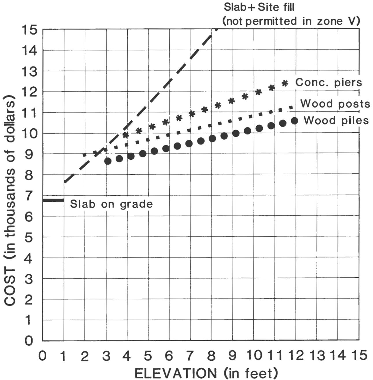
Figure 5.5. Relative Costs of Foundations Elevated to Different Heights
