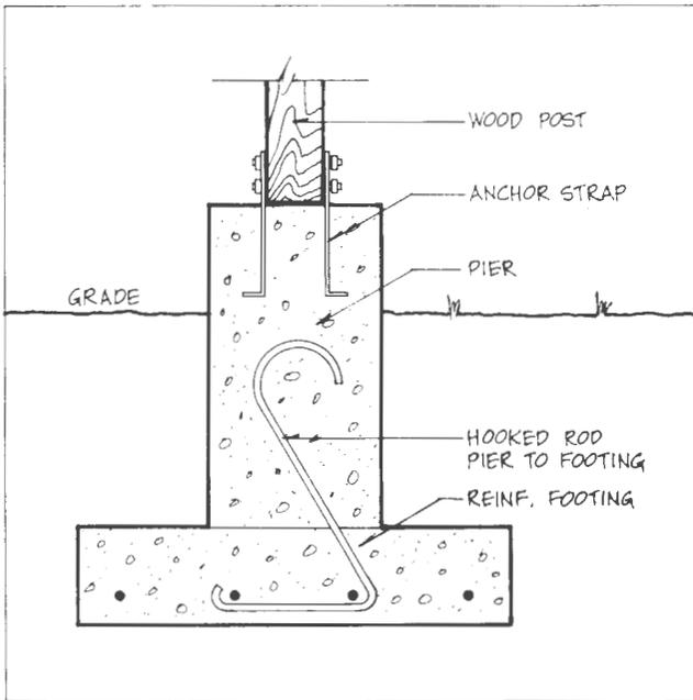
Figure 4.9. Post/Pier Foundation
