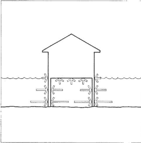
Figure 2.1. Hydrostatic Forces
