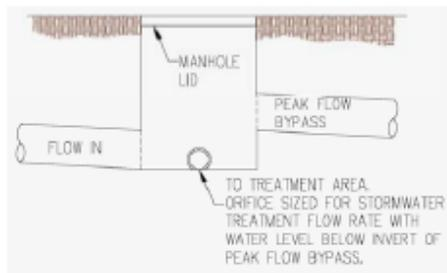
**Figure 4-14: Stepped manhole design directs low-flows to treatment measure and diverts high flows to storm drain system. (BKF Engineers)**
