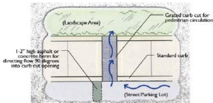
Figure 4-13: Grated curb cut: plan view (Source: SMCWPPP 2009)
