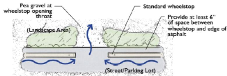
Figure 4-10: Opening between wheelstop curbs: plan view (Source: SMCWPPP 2009)
