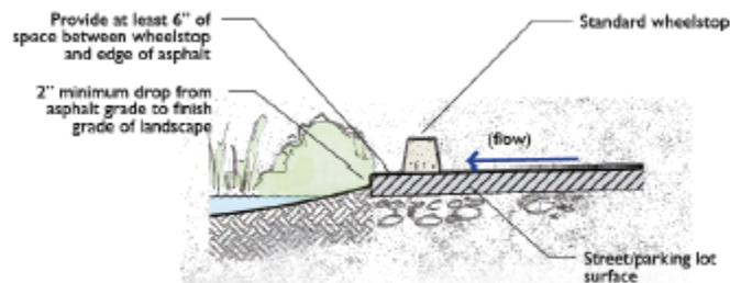
Figure 4-9: Opening between wheelstop curbs: section view (Source: SMCWPPP 2009)
