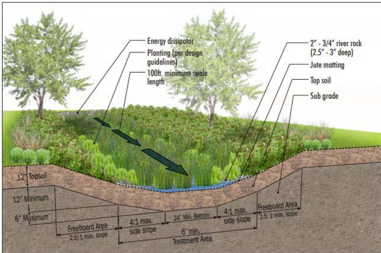
Figure 3: Typical Design and Structure of a Vegetated Swale (from Clean Water Services)
