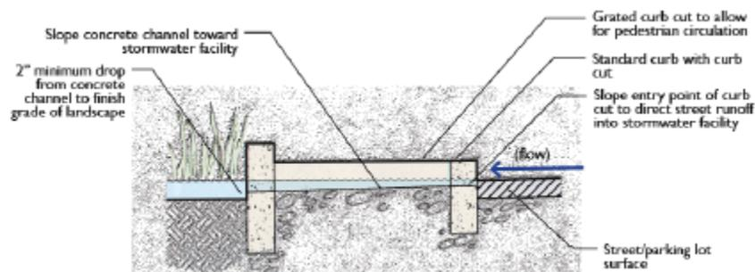
Figure 4-12: Grated curb cut: section view (Source: SMCWPPP 2009)
