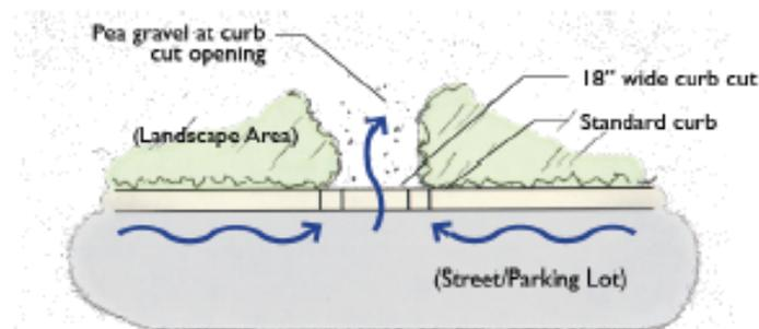
Figure 4-4: Standard curb cut: plan view (Source: SMCWPPP 2009)
