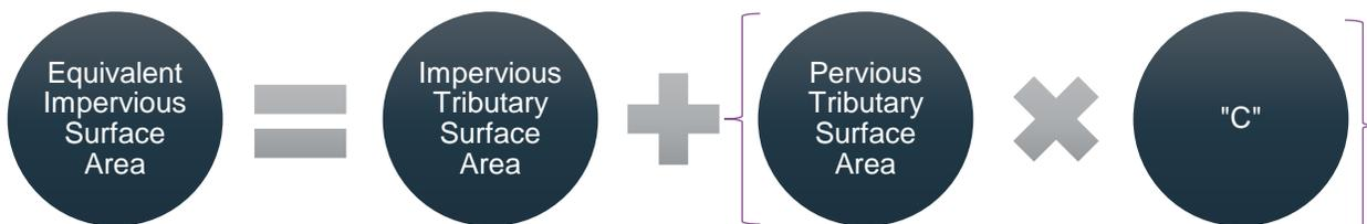
**Figure 11. Equivalent Impervious Surface Area Equation**
