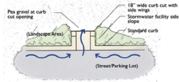
Figure 4-7: Standard curb cut with side wings: plan view (Source: SMCWPPP 2009)
