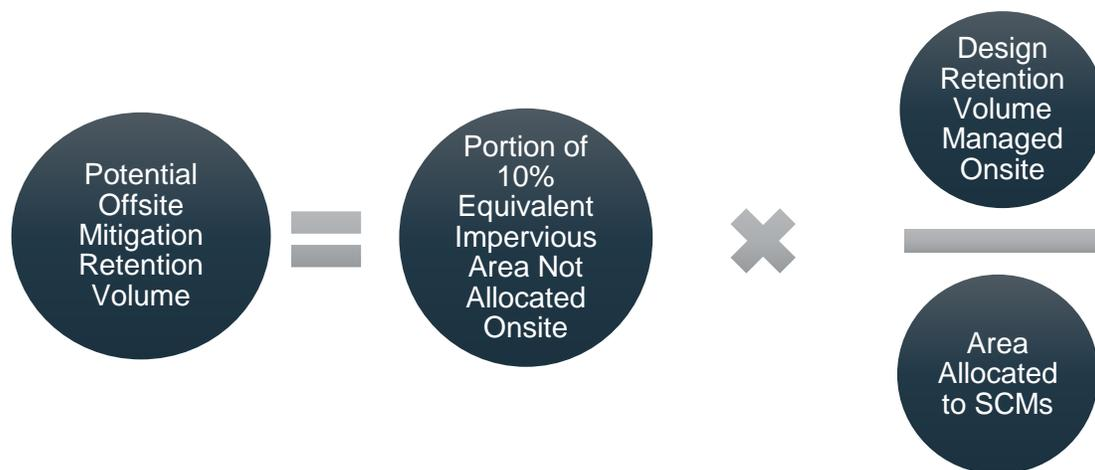
**Figure 12. Potential Offsite Mitigation Retention Volume Equation**
