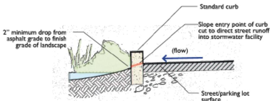
Figure 4-3: Standard curb cut: section view (Source: San Mateo Countywide Water Pollution Prevention Program [SMCWPPP] 2009)
